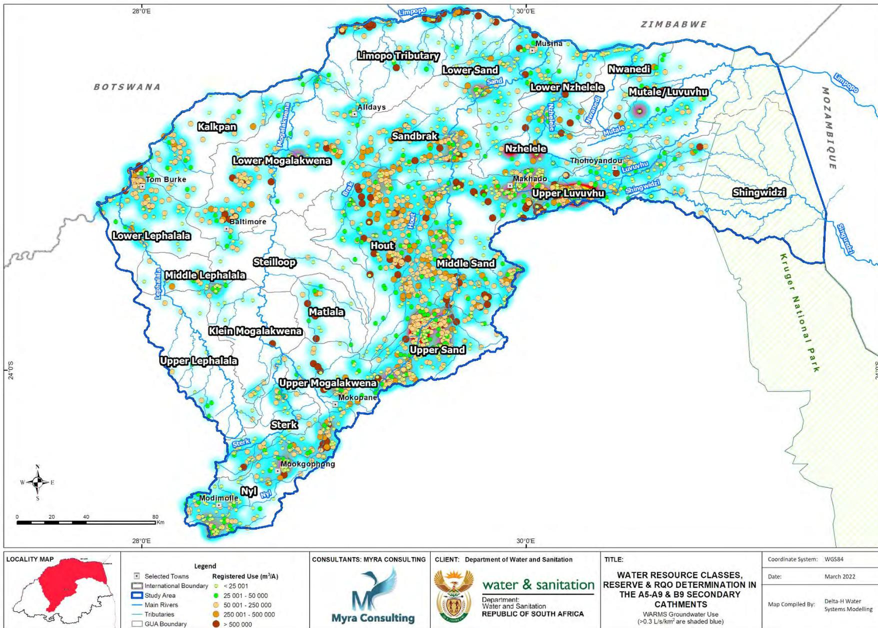
Figure 13. Map showing distribution of registered groundwater abstraction (points) and groundwater use >0.3 L/s/km<sup>2</sup> shaded.
