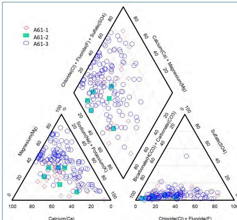
**Figure 20. Piper diagram for the Nyl and Upper Mogalakwena drainage region.**
