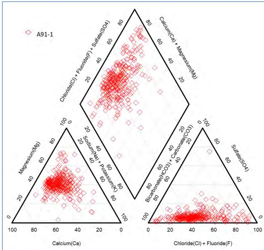
Figure 42. Piper diagram for the Upper Luvuvhu drainage region.
