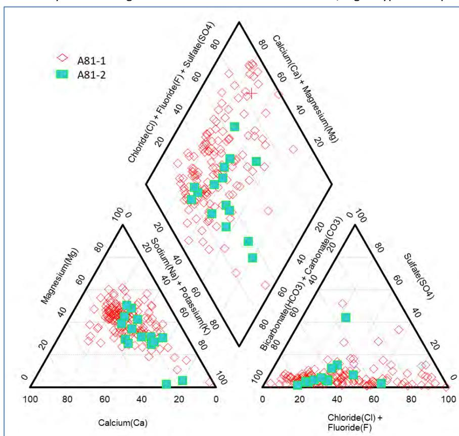
**Figure 37. Piper diagram for the Nzhelele drainage region.**
