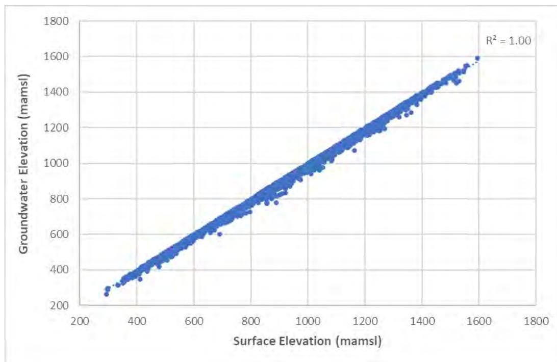
**Figure 8. Correlation between surface topography and groundwater elevations for the study area.**
