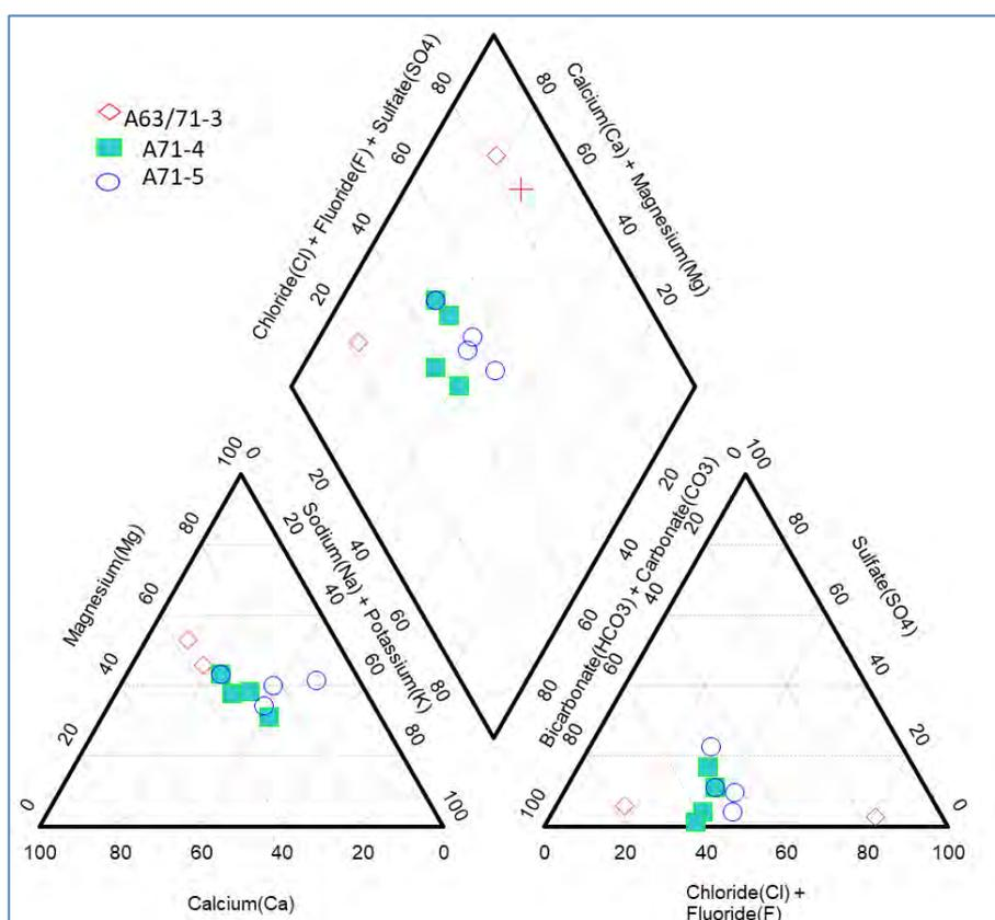
**Figure 33. Piper diagram for the Lower Sand and Limpopo Tributary drainage region.**
