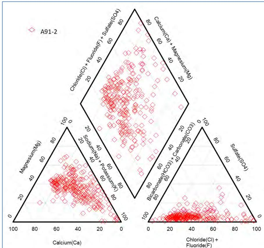
Figure 44. Piper diagram for the Mutale/Lower Luvuvhu drainage region.
